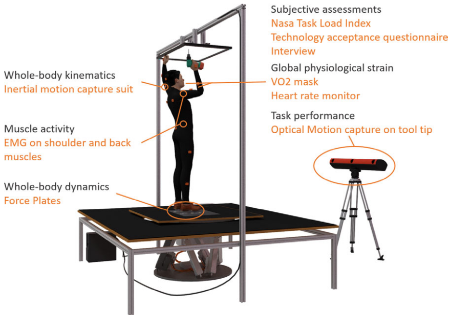
Figure 2. Experimental set up for data recording at the laboratory experiment.
