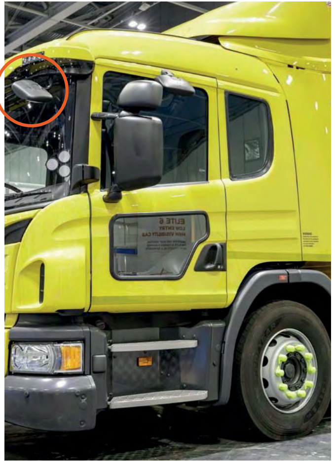
Class VI mirror shall be fitted to the front of the vehicle
