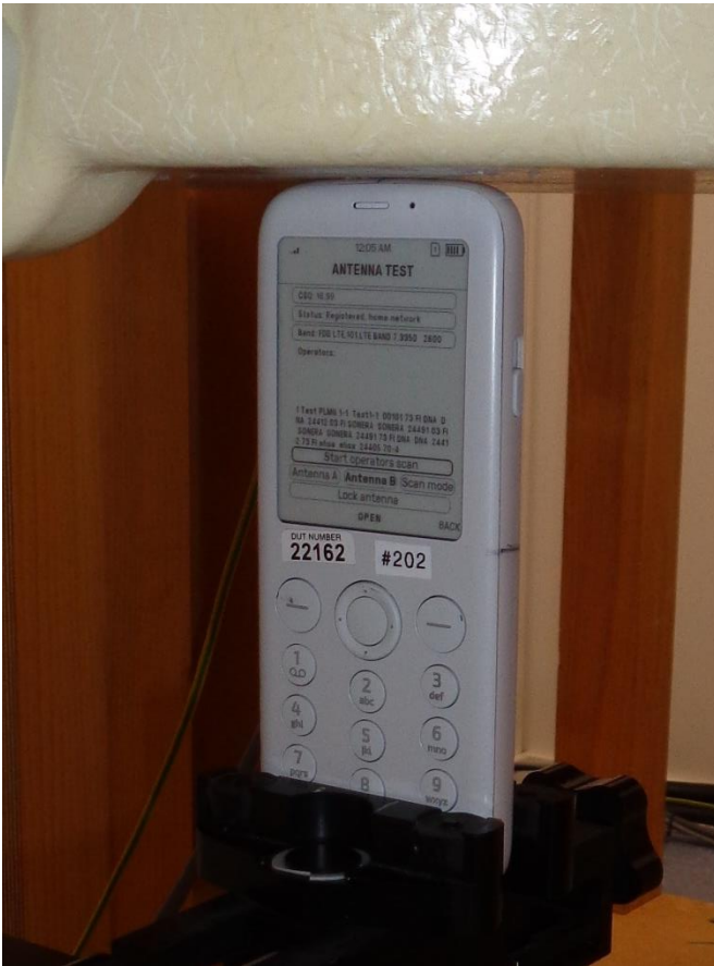
Limb configuration, top side towards the phantom with 0mm separation.
