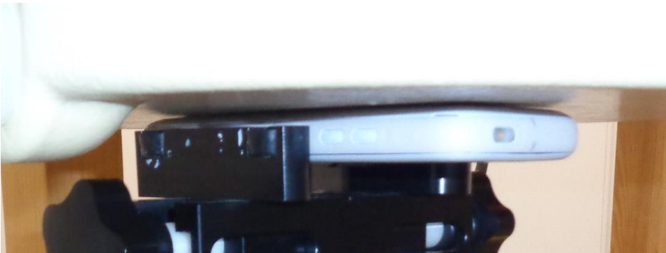
Limb configuration, back side towards the phantom with 0mm separation.
