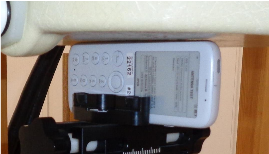
Limb configuration, left side towards the phantom with 0mm separation.
