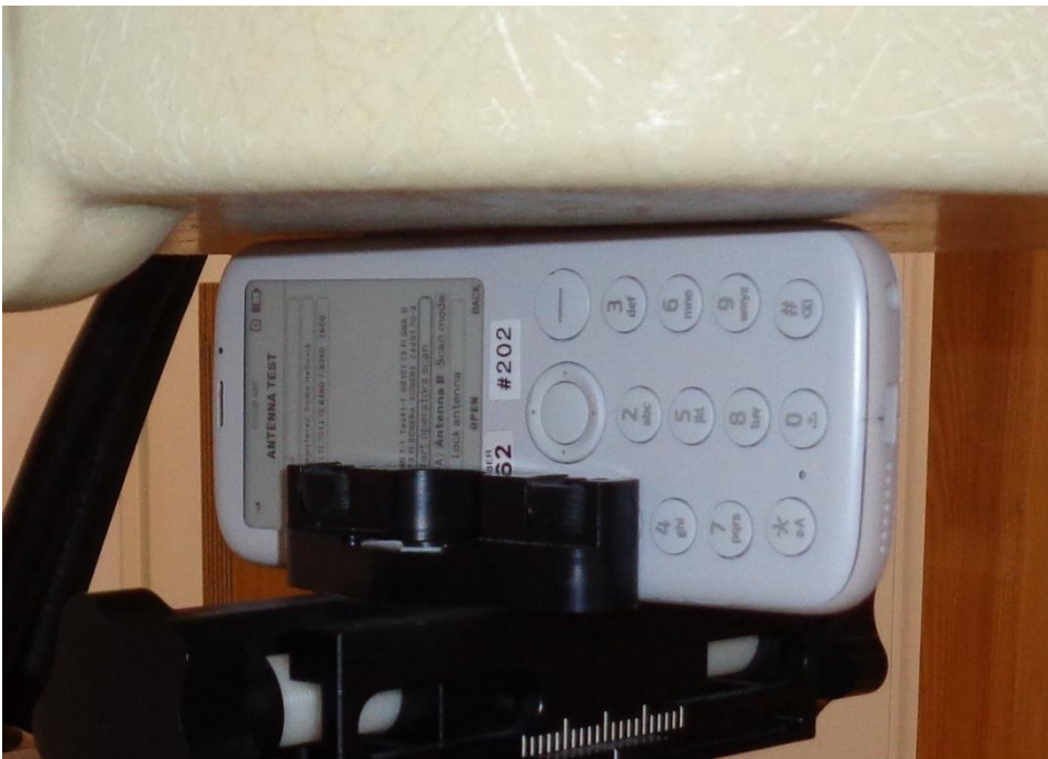
Limb configuration, right side towards the phantom with 0mm separation.
