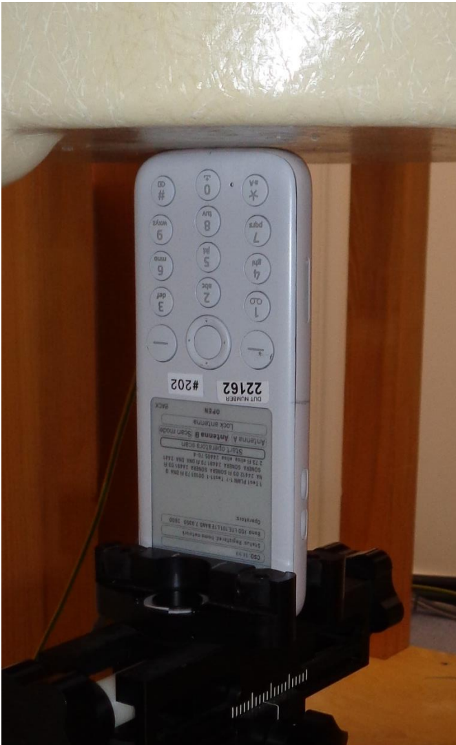
Limb configuration, bottom side towards the phantom with 0mm separation.
