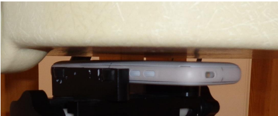
Body-worn configuration, back side towards the phantom with 5mm separation.
