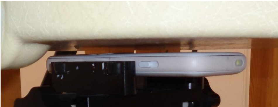
Body-worn configuration, front side towards the phantom with 5mm separation.
