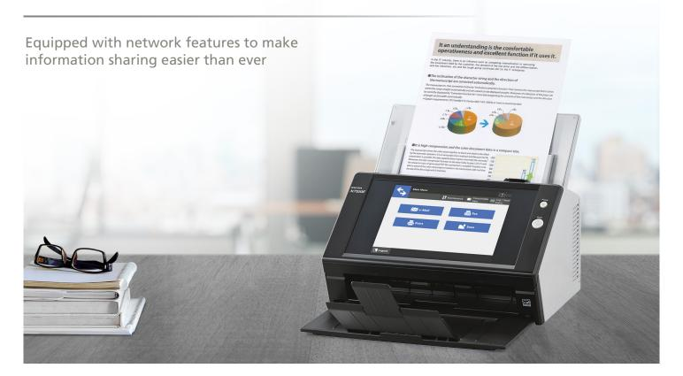
The N7100E is an easy-to-use shared, stand-alone network scanner with a large touch screen and job buttons to make distributed work flows more efficient. Scanning speeds are a consistent 25 ppm/50 ipm (A4 landscape 200/300 dpi) with a 50 sheet loading capacity.
