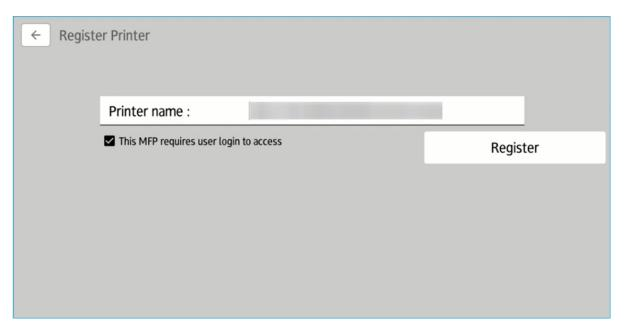
"This MFP requires user login to access" is displayed below the printer name field. If this is checked when **Register** button is pressed, a dialog is displayed requiring Printer Admin to enter the machine admin credential. If "This MFP requires user login to access" is unchecked, please skip the next step.
