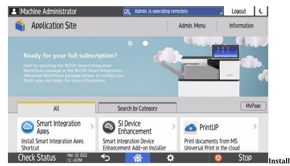
**from WIM** – If unable to install from Application Site, you can try installing from the device WIM.
