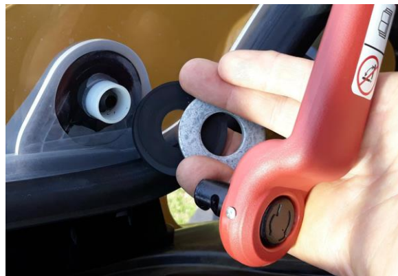
Figure 5 - This image shows the correct relationship of the inner components of the lower handle assembly. Note the rubber washer is next to the window and the steel washer is next to the handle. The lower handle components are assembled in the same order as that shown in Figure 3 for the upper handle.
