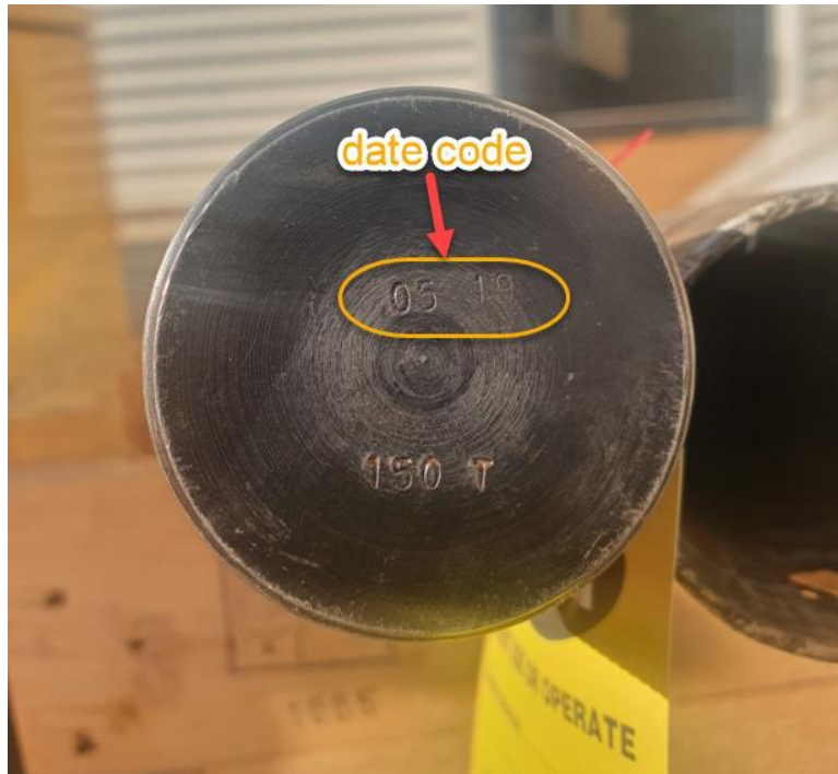
Figure 1 - Date code '05 19' found on 9U-7763 puller studs to be removed from use.
