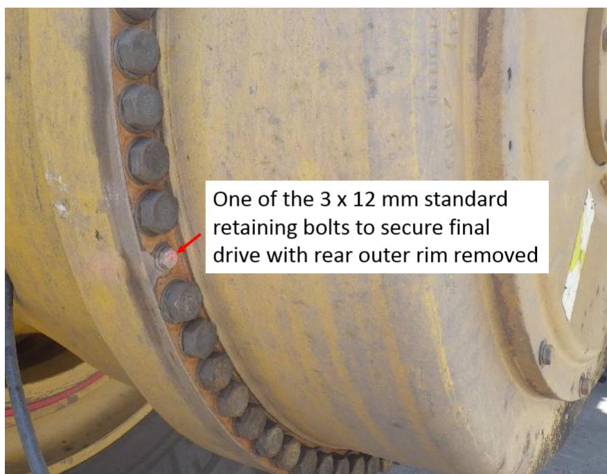
Figure 1 - Shows correct installation of shorter bolts with hardened flat washer, typical of 785 - 793. (793F shown)
