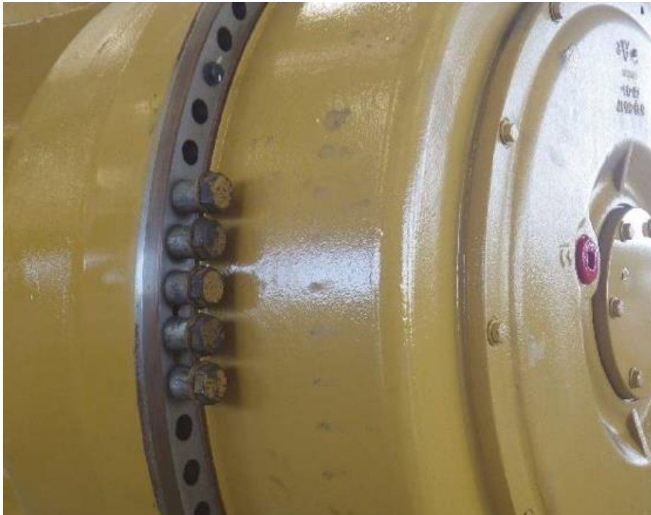
Figure 2 - Shows insufficient bolts with unsuitable spacers – requires installation of all bolts with spacers similar ID and OD as flat washers with parallel (machined) end faces. (793F shown)
