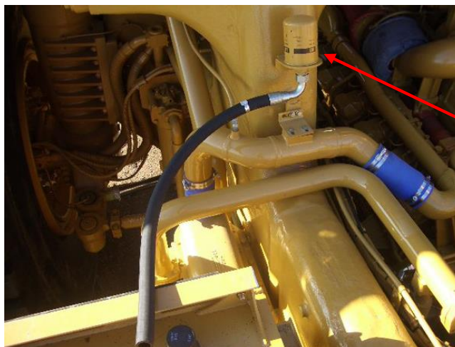
Typical location of fuel tank breather - 797B shown
