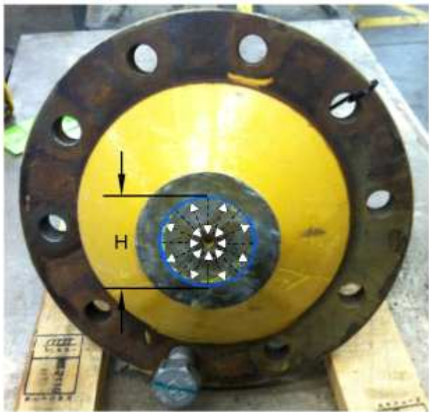
Illustration 3 g06040021 Scan Pattern and Area (H) Diameter of Scan Area Ø 70.0 mm (2.75 inch) 14 and Ø 80.0 mm (3.15 inch) for 16 and 18 models Inspections can be conducted on built machines with no need to disassemble and remove front spindles.
