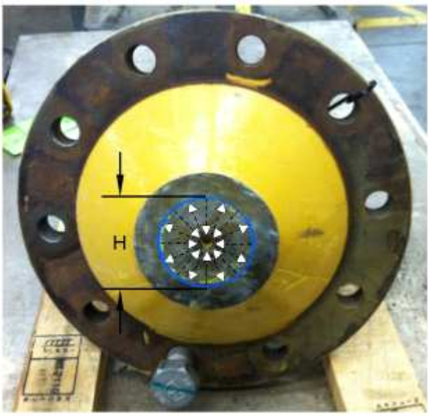
Illustration 8 Scan pattern and area (H) Diameter of scan area 80 mm (3.15 inch)
