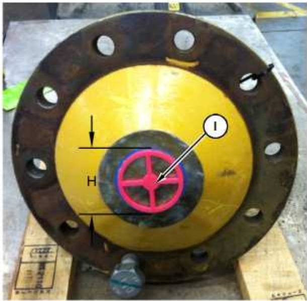
Illustration 2 g06039999 (H) Diameter of Scan Area Ø 70.0 mm (2.75 inch) 14 and Ø 80.0 mm (3.15 inch) for 16 and 18 models (I) Outline Marking Template
