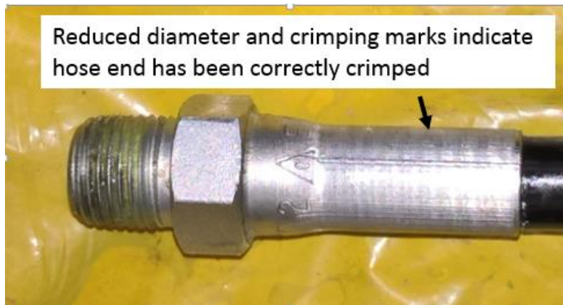
Illustration 2. Correctly crimped fitting – no action required.
