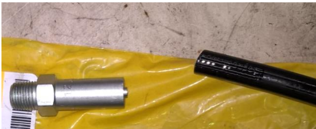
Illustration 1. Hose separated from fitting due to missed crimping process during manufacture.
