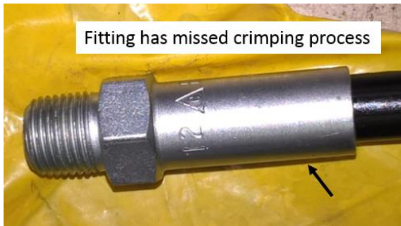
Illustration 3. Fitting has not been crimped – Do not use.
