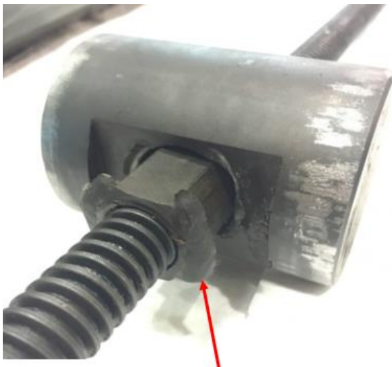
Failed weld connecting nut to pin
