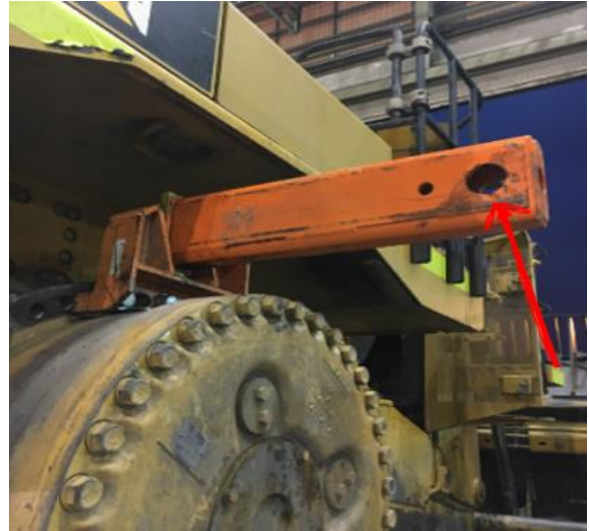
Sliding section - bracket removed showing pin location
