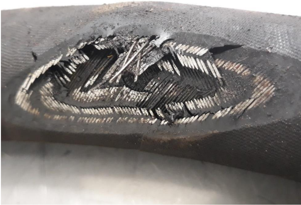
Illustration 1. Hose has worn to the point of failure.
