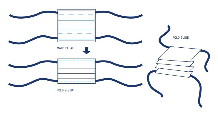
**BEFORE YOU CUT FABRIC:** You need to cut out both Mask A1 and Mask A2 for this pattern, then combine them by butting them up (DO NOT OVERLAP) and taping them together. The final pattern piece is 9 inches long by 9 inches wide. See diagram on next page.
