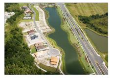
Estancia at Wiregrass – The project consists of over 700,000 cubic yards of excavation, over 3 miles of roadway construction, a new lift station, and 100,000 LF of various utility pipe.
