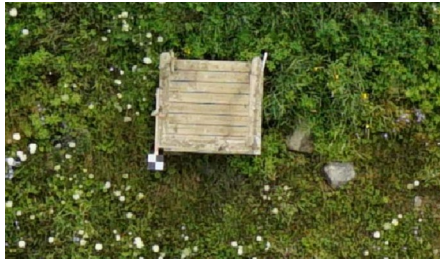
Figure 4. Photo identifiable metal checkered target affixed to wooden structure
