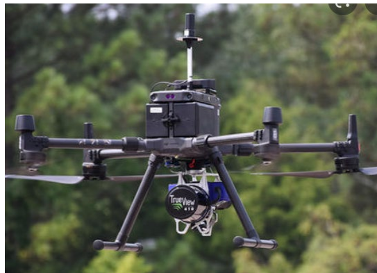
Figure 14: TruView 410 on M300 UAV
