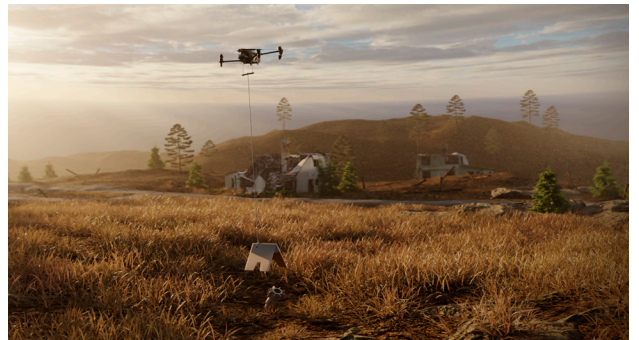
1. Transport the clearing charge using a drone.
