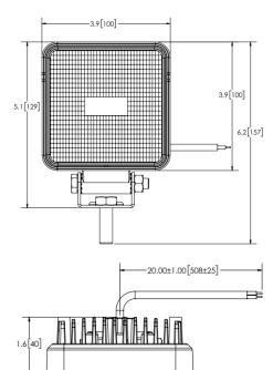
E92007-MG is supplied with 15' cable and 15" pigtail connector
