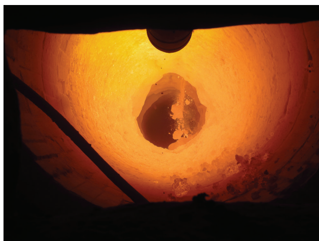
Figure 2. Formation of Solidia clinker nodules in a rotary kiln heated to 1200 °C.
