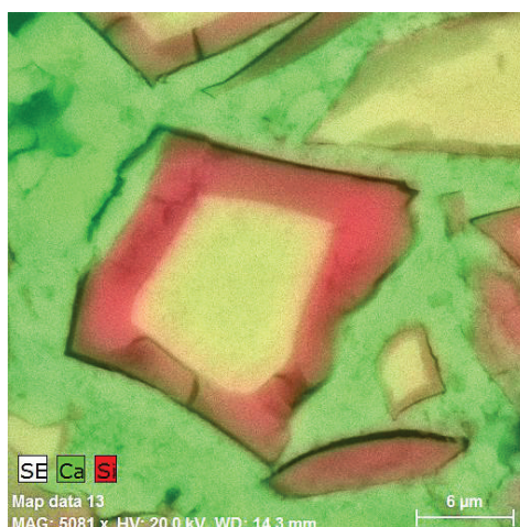
Figure 4. Microstructure of CO 2 -cured Solidia cement: the green area is calcite (CaCO 3 ), the red area is amorphous silica (SiO 2 ) and the yellow area is unreacted wollastonite (CaO·SiO 2 ).
