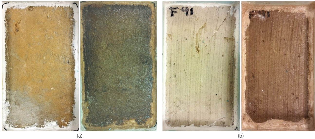
Figure 4. OPC-C (a) and CSC-C (b) specimens before and after completion of 50 freeze–thaw cycles in scaling tests
