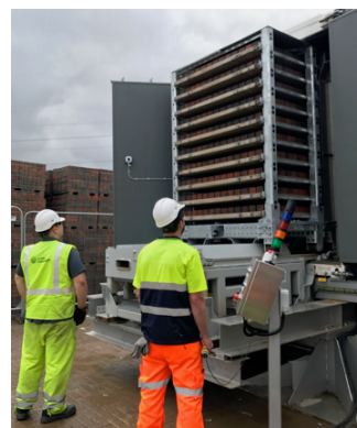
Figure 2: Solidia Technologies' curing chamber installed at a UK precast site
