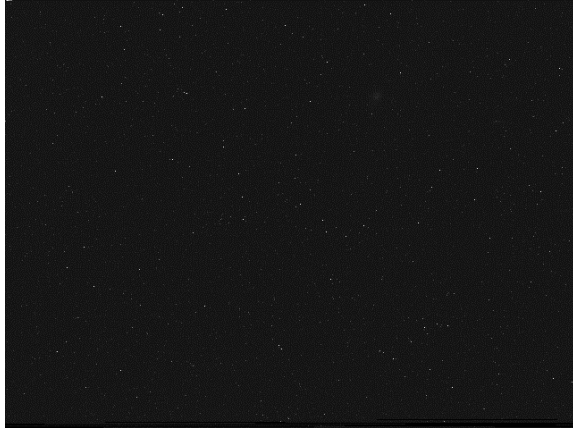
Figure 11: An un-processed ELSA-d VISCAM exposure displaying numerous hot pixels. At first glance they look like stars, but are recognisable from their sharpness and constant position throughout image sequences.
