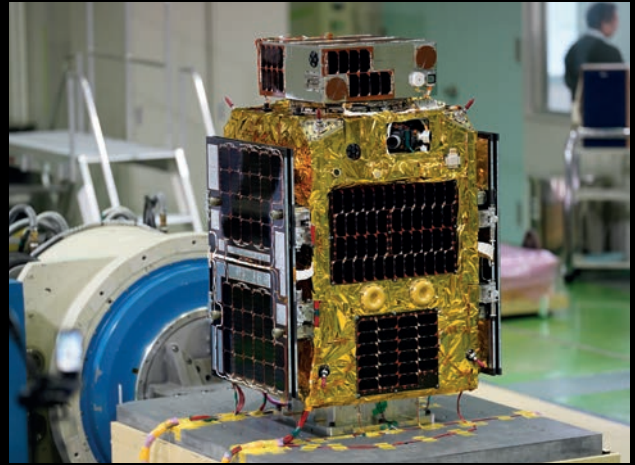
Vibration testing at JAXA's Tsukuba Space Center in February 2020
