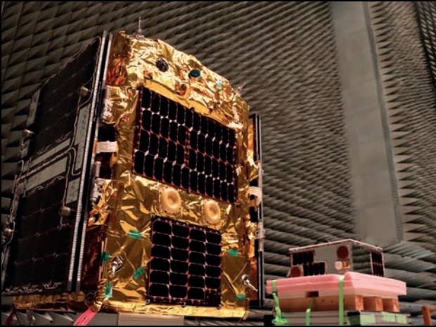
Electromagnetic compatibility testing in February 2020
