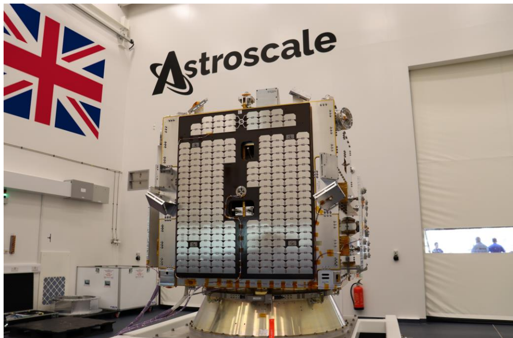
Fig. 3. ELSA-M SQM following integration in Astroscale's clean room, prior to shipment for testing
