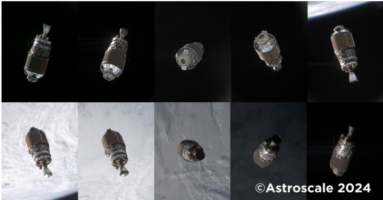
Fig.12: Client image captured by the fly-around observation #1
