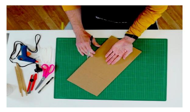
Using a marker or pen, draw the design for your robot hand. Trace a rough rectangle around your actual hand, which will become the wrist of the robot hand.
