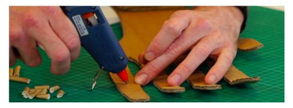
Using the hot glue gun, stick the shorter pieces of straw vertically in the middle of the finger, between each bend. Glue the longer pieces to the palm like a fan.
