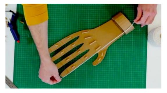
Use one piece of string per finger, thread the string through the straw pieces. Make sure that the top of the string reaches the tip of the finger and the bottom of the string reaches the wrist.
