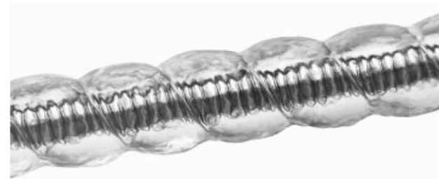
A magnified view of the hydrogel-coated coil.
