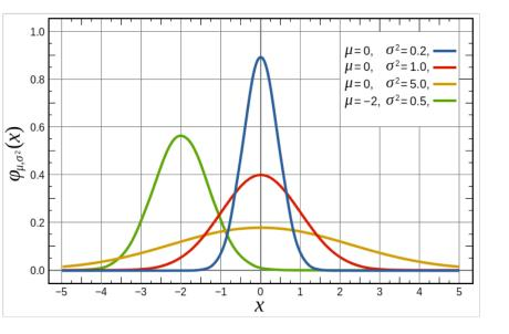
Notice: value of the normal distribution approaches zero when x is more than a few standard deviations away from the mean
