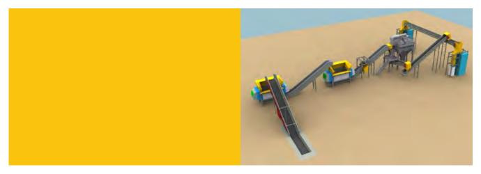
If a more refined shred is needed, a horizontal incline conveyor can pass the pre-shredded material through to a secondary machine such as the new UNTHA XR3000XC, to achieve a more precise <20mm fraction.
