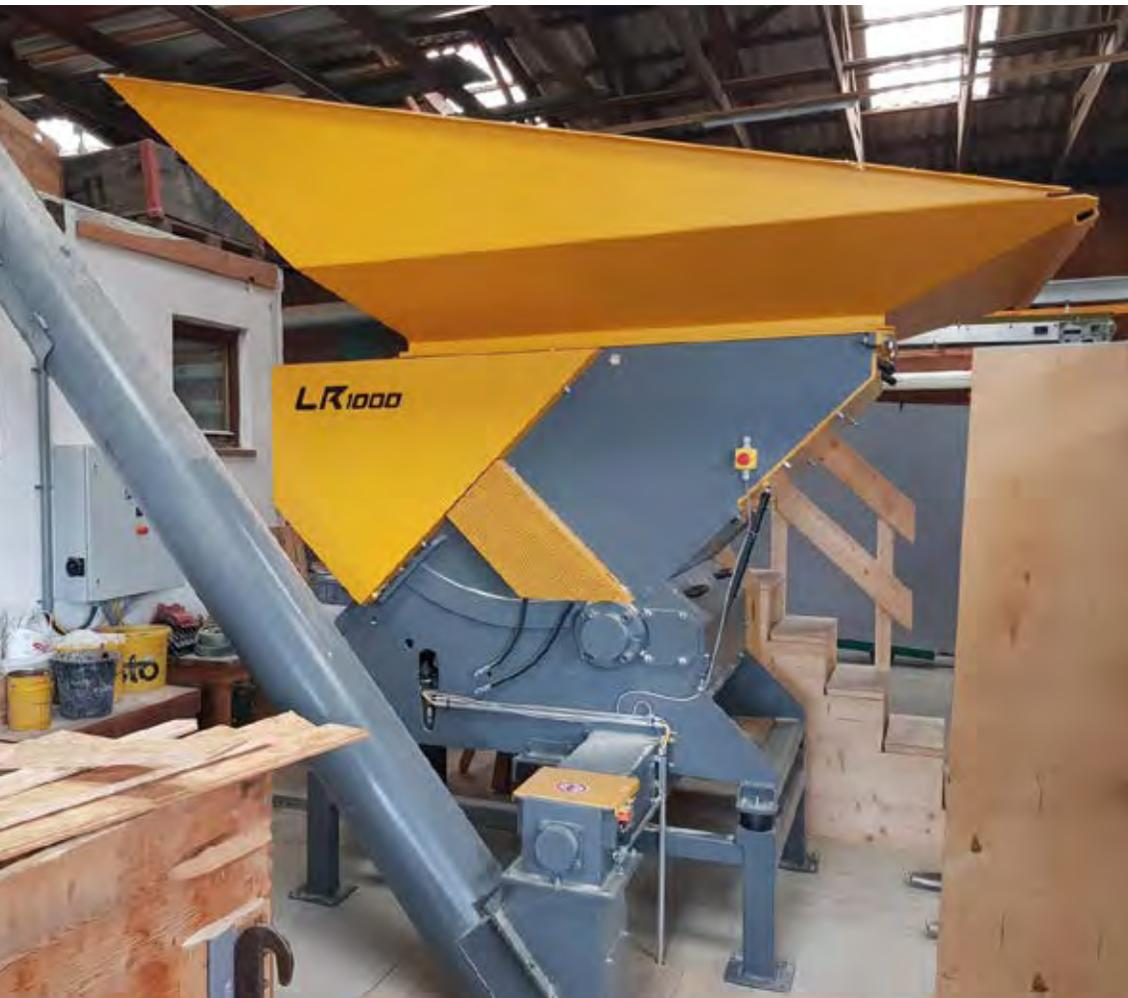
Holzbau Gerstenmayer is a timber construction company based in Karlstetten in Lower Austria. Business has grown steadily in recent years, as have the company's residual wood volumes. For this reason, the company has invested in an LR1000 shredder by UNTHA shredding technology.
