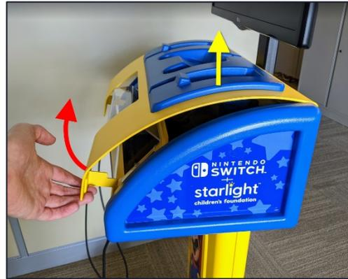
4. Use a 7/16" socket driver to remove the two nuts that attach the console cover assembly to the cabinet. Once the nuts are removed, lift the console cover assembly way from the cabinet and set aside for reinstallation later.
