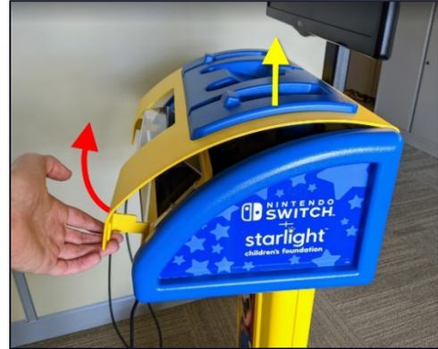
4. Use a 7/16" socket driver to remove the two nuts that attach the console cover assembly to the cabinet. Once the nuts are removed, lift the console cover assembly away from the cabinet and set aside for reinstallation later.
