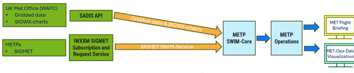
Figure 11. An example of approaches that MET ANSPs could take to consume the En-route and Approach Meteorological Information service
