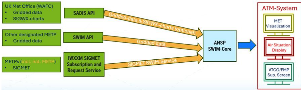
Figure 10. An example of approaches that ATS ANSPs could take to consume the En-route and Approach Meteorological Information service
