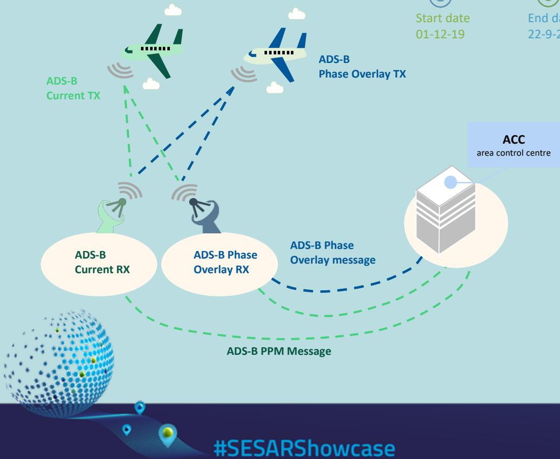
PJ.14-W2-84d is a **technological solution validating new ADS-B communication link, Phase Overlay**, enabling the transmission of extra information, complementing the current ADS-B PPM with an 8PSK phase modulation.
