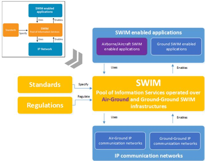
Flexible airborne SWIM infrastructure deployment enables to “SWIMIZE” current and future Air Traffic Services (ATS) and Aeronautical Operational Control (AOC) communication bringing benefits in terms of reliability, security, interoperability, agility and air-ground network resources usage.
