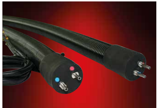
ELH/2aw-200 °C-NW6, analytic hose with 2 inner liners NW 6/8 made of PFA with transition-free special RSL pipe stub on both sides. Holding temperature 200 °C
