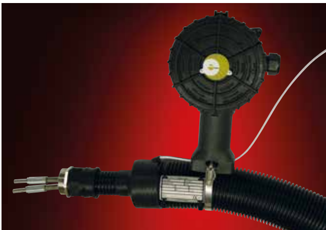
Special analytic heated hose type ELH/2adsbw-100 °C- NW6/8-EX-SP for ex-range with 2 inner liners made of PTFE NW 6/8 and attached Ex terminal box; type Ex-it-R. Holding temperature: 100 °C
