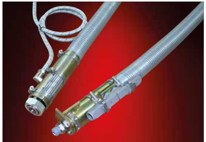
ELH-hdT 200 °C, NW 16 Heated pressure hose featuring tread-resistant design with corrugated metal hose as outer jacket, additional wire and special end cap; Application: Bitumen technology
