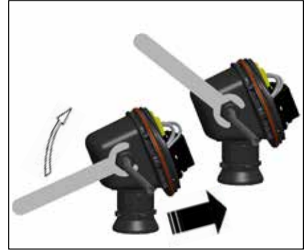
2. Remove M25 dust cap. Install M25 gland (order separately) blind plug. Install power/control cable.
