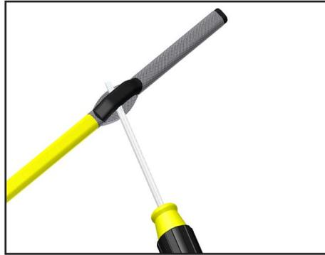
2. Separate braid strands at edge of overjacket and pull cable through opening in braid.
