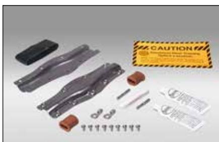
SK-SX-OJ... Ex e approved under-the-insulation repair and splice kit for overjacketed SX cables. Kit includes stainless steel shells, screws, grommets, RTV adhesive/sealant, insulation tape and the necessary wire pins/lugs.
