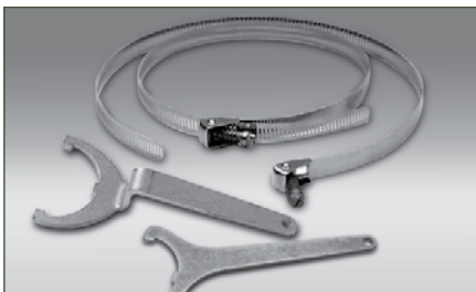
B-4, B-10, B-21... stainless steel attachment bands for securing Thermon nonmetallic kits to pipes. B-4... for pipes up to 100 mm diameter B-10... for pipes up to 250 mm diameter B-21... for pipes up to 530 mm diameter ABA-25... for pipes up to 25 mm diameter ABA-40... for pipes up to 40 mm diameter Terminator-LN-Tool... for tightening the locknuts of the Terminator kits. Tool is recommended to ensure enclosure is properly secured to the pipe-mounted expediter.
