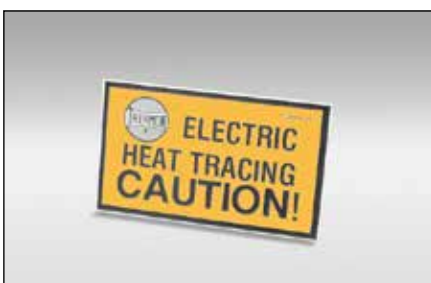
CL... vinyl-based peel-and-stick caution labels are intended for direct exposure to industrial environments. Electrically heated pipelines and vessels should be clearly identified at frequent intervals along the pipeline or vessel. Caution labels should be placed at 3 to 6-m intervals or as required by code or specification. Additional languages or other texts are available; contact Thermon.
