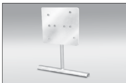
XP-1... predrilled stainless steel (type 304) mounting bracket designed for mounting Thermon junction boxes and thermostats directly to the pipework. The bracket is easily secured to the pipe using B-4, B-10 or B-21 attachment bands. The XP-1 utilises a 110-mm standoff.
