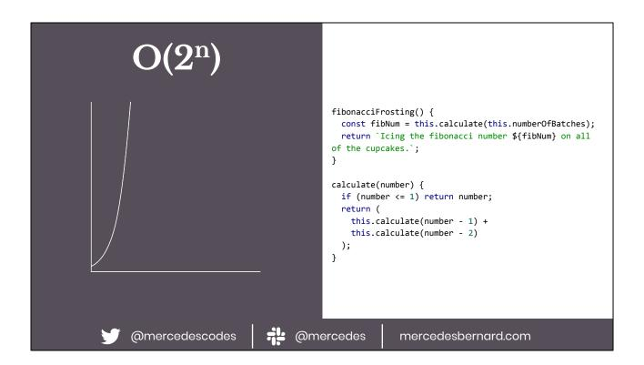
$O(2^n)$  = Running time grows exponentially with the size of the input. For example, calculating Fibonacci recursively
