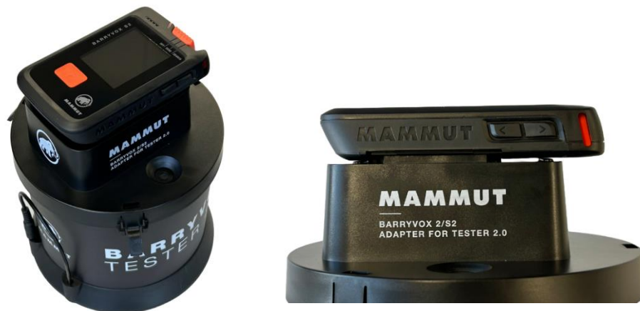
Figure 1 Connecting the adapter to the tester 2.0
