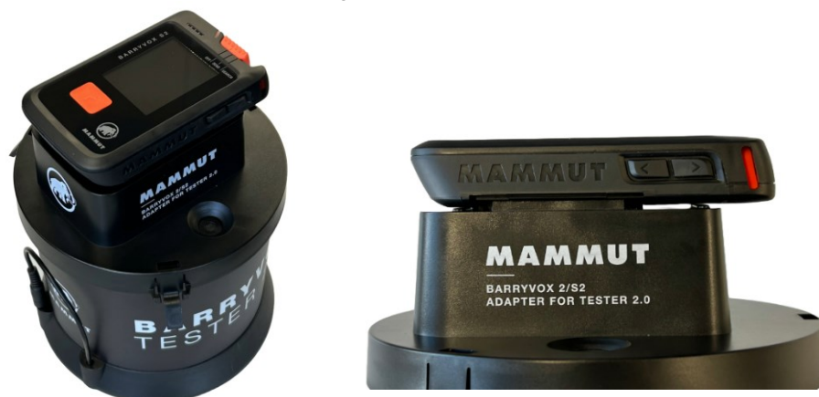
Figure 1 Connecting the adapter to the tester 2.0
