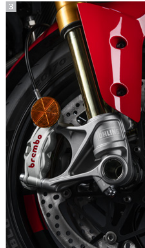
3 Electronic Öhlins Smart EC 2.0 suspension
