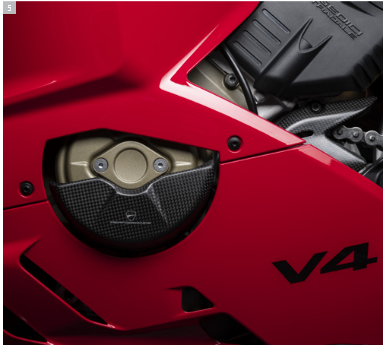
5 Carbon protection for generator cover.
