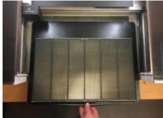
**4** Slide in the Crumb Tray. Slide it in until you feel the feet settle into the dimples in the base of the Glowforge unit.
