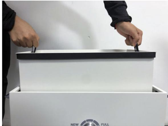
*Lift the filter cartridge out*
