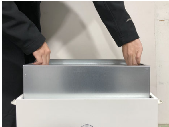
Lift the filter cartridge out
