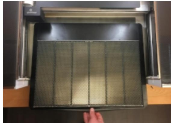
**4** Slide in the Crumb Tray. Slide it in until you feel the feet settle into the dimples in the base of the Glowforge unit.
